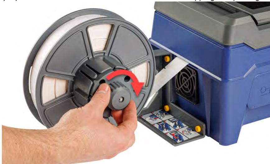
21. Tap **Feed Supply** on the touch screen to advance the label supply. You may need to tap several times until a label dispenses from the printer.
