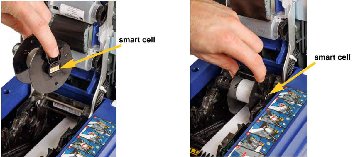
18. Make sure the labels below the core are aligned between the disks on either side of the core.
