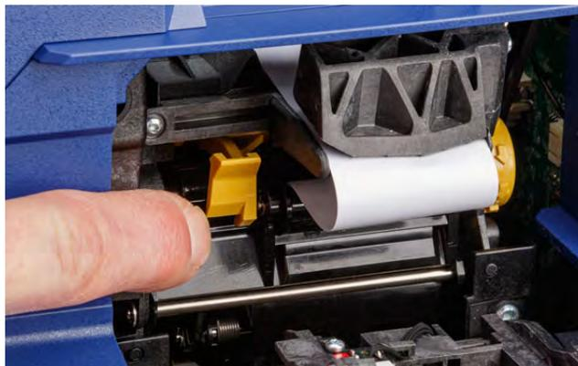
12. Turn the thumbwheel to the right of the peeler to tighten the liner.
