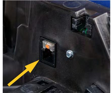
5. Clean the **ribbon out sensor** in the printer chassis with a clean swab dipped in isopropyl alcohol.
