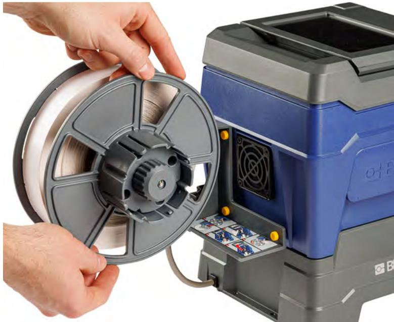
7. Feed the labels through the slot in the back of the printer, just above the fan.
