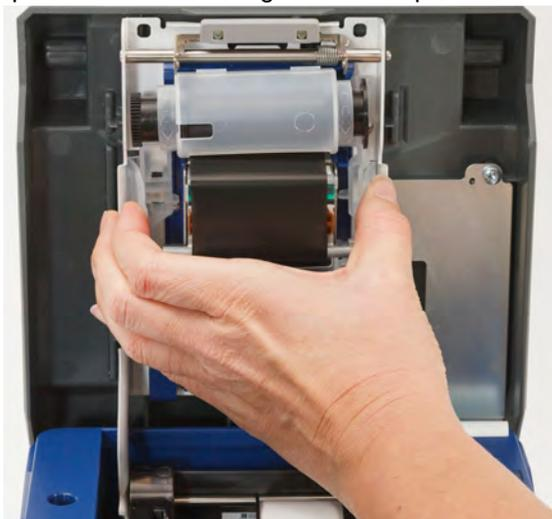
If the ribbon is spent, recycle the cartridge according to local regulations. If the ribbon is not spent, store it in a cool, dry place. Unused ribbon will last up to six months before deterioration sets in.
