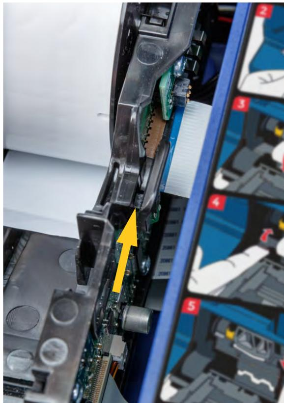
6. Clean the smart cell contact in the top cover with a clean swab dipped in isopropyl alcohol.
