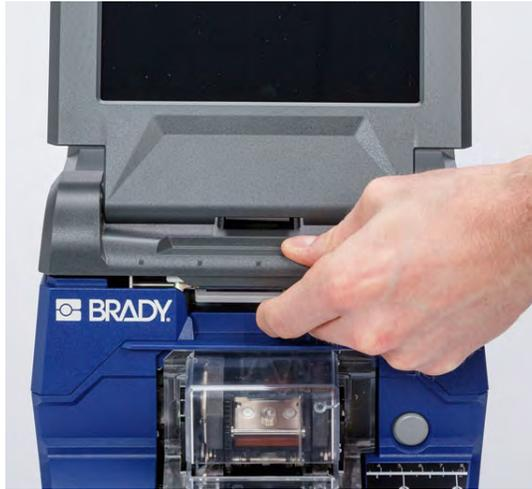
3. Remove the currently installed label roll. Note the correct placement of the label supply before removing it.
