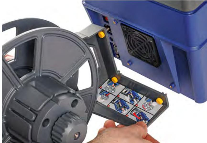
2. Insert and tighten the three thumb screws.
