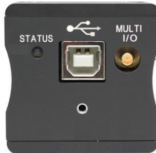
Figure 2.1 USB Connector and Status LED
