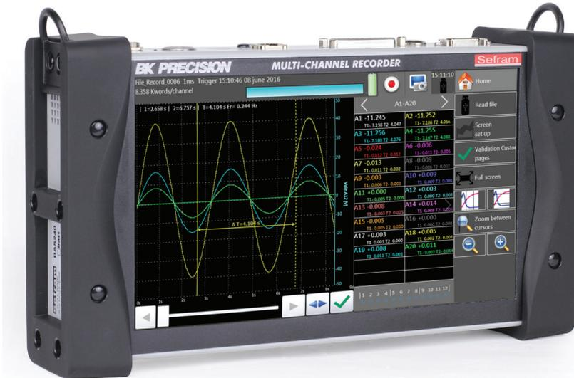
The DAS240 is ideal for measuring and recording common parameters such as voltage, current, temperature, pressure, and more with sampling rates up to 1,000 samples per second. It includes 20 universal analog inputs with convenient screw terminals, and an expandable design to support up to 200 channels. This data logger also provides digital inputs and alarm outputs for process monitoring applications.
