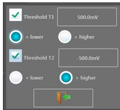
Figure 9.5 Alarm Analog Thresholds
