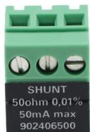
The 50  $\Omega$  shunt can be used on any channel of the recorder to accurately measure, display, and record the output from 4 to 20 mA current loop sensors.
