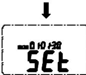
1: press and hold the "A/C" button and then power on the meter:
