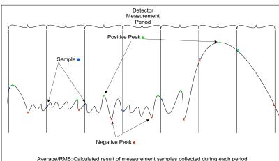
Figure 14 Detector Operation
