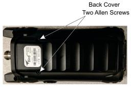
4. Disconnect battery connector from chassis. See Figure 34.
