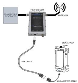
Figure 32 Power Sensor Connections
