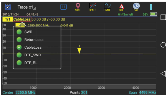
Figure 30 Selecting Cable Loss Measurement
