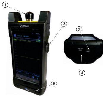
Figure 1 SK-6000 Controls, Indicators, Connectors and Ports
