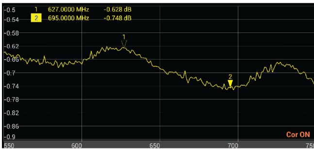
Figure 11 Interpreting Cable Loss Measurement
