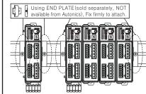
**※Make sure to install the unit vertically** to the ground.
