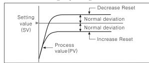
\*\*Manual reset function is applicable only to P / PD control mode.
