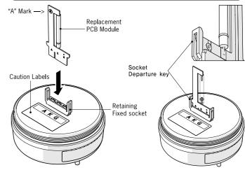
The new lamp should be inserted firmly to match the same signal A K G (or A G K) mark. Printed "A" in circuit and label.
