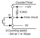
**%CP1**, CP2 (INHIBIT), RESET input part
