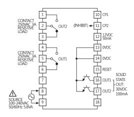
※INHIBIT: In case of timer mode, this terminal is for time hold. (voltage input (PNP): connect with 12VDC, no-voltage input (NPN): connect with 0VDC)
