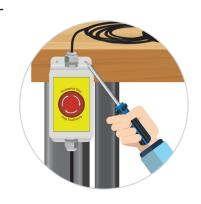
**Step 2** Connect female end of E-Stop to the instrument you wish to control.
