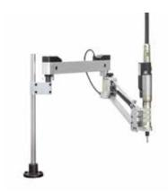
The Tracer Arm for the EH2 vastly improves operating efficiency and ensures error-proof assemblies. It is equipped to detect the position of the EH2 tool and compare it to preprogrammed position data. The operator must perform the fastening sequence properly or the tool is disabled. Fastening data is stored and can be exported for qualification and analysis.
