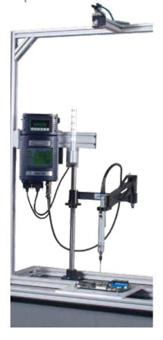
The sequence recognition system is the solution for applications such as those requiring uniform compression of all components within your product assembly. The ASG SRS ensures that the operator installs fasteners in a specific pre-programmed sequence.
