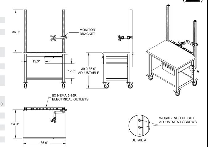
All dimensions are in inches unless otherwise specified. All dimensions have a tolerance of  $\pm 0.5$ " unless otherwise specified. Specifications and procedures are subject to change without notice.
