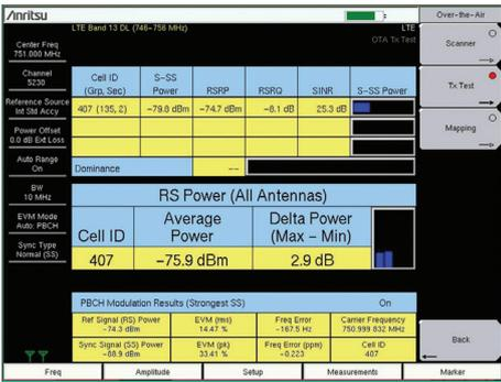
**Over-the-Air Measurements – Tx Test**
