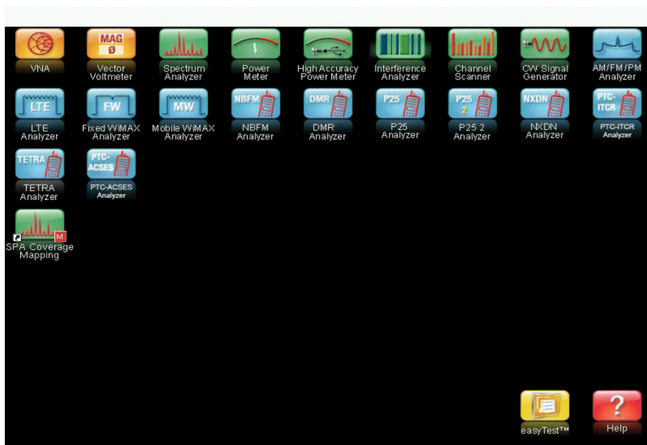
Figure 2-2. Menu Key Screen, Icons for Installed Measurements
