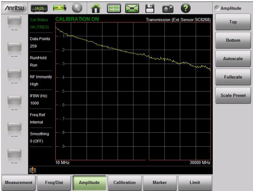
Figure 3-15. External Sensor Transmission Measurement Example
