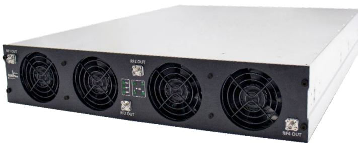
Figure 4: APVSGXX-4 in a 2U case
