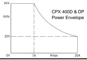
The power envelope is set to give 60V/7A, 42V/10A and 20V / 20A under all supply conditions (both outputs loaded); at lower output voltages the output power is restricted by the 20A current maximum.
