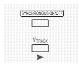
The SYNCHRONOUS ON/OFF key is in addition to the individual OUTPUT switches and permit both outputs to be turned on or off synchronously with a single key press. Since this key turns both outputs on or off with alternate presses it is necessary for both outputs to be in the same state (i.e. both on or both off) before the key is used. Pressing the key with one output on and one output off will have no effect.
