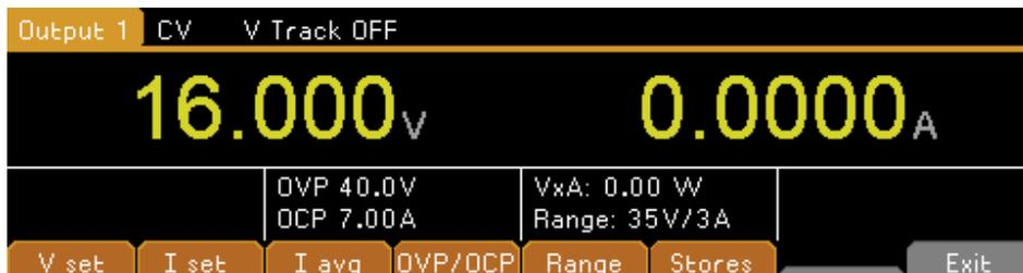
The top line shows the operating mode (CV, CC or SET) together with the voltage tracking status. The meters are displayed in a larger font, and the complete settings status for the output is shown below them.
