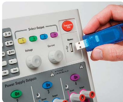
Figure 12. The N6705's front panel USB port.
