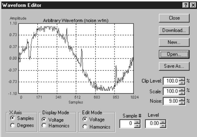
Figure 6. User defined waveform: noise with spikes
