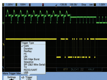
Trigger on and decode CAN serial packets.
