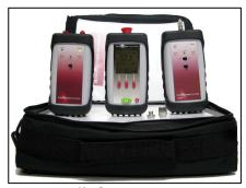
designed for both multimode and single-mode applications. The AF-OLK5N<sup>NextGen</sup> series test kits come with the AF-OM120N-I series power meter. The meter is accompanied with the AF-OS420N 850/1300nm LED light source for multimode applications or/and AF-OS430N 1310/1550nm laser source for single-mode applications (AF-OS430N comes equipped with interchangeable ST, FC and SC connector adapters).
