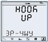
Hook up, voltage and current ratios and aggregation period can be configured from the front panel of the PEL 103.
