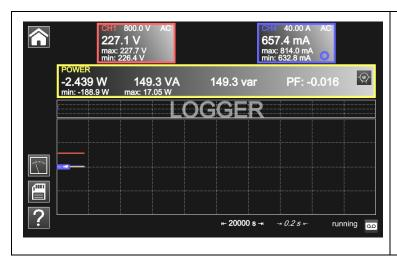
Each recording file contains 100,000 measurements per channel, at a rate of one measurement every 0.2 sec for 20,000 sec (approx. 5h30').
