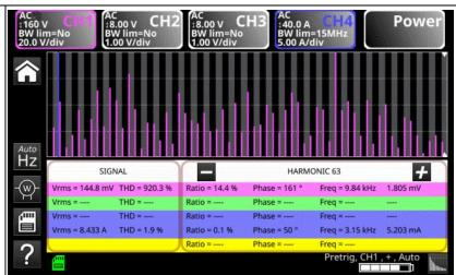
The measurement parameters displayed: Signal Measurement
