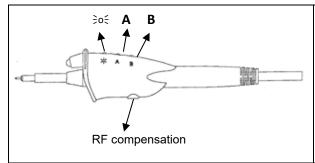
The *HX0030* probe has three directly accessible control buttons:
