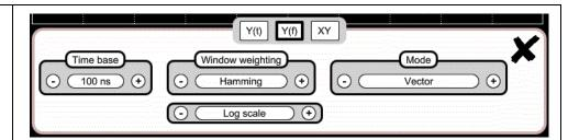
The *Fast Fourier Transform (FFT)* is used to calculate the discrete representation of a signal in the frequency domain from its discrete representation in the time domain. It is calculated on 2500 points. It can be used in the following applications:
