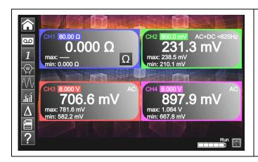
Channel 1 of the *ScopiX* is named CH1. It measures various physical quantities in addition to the signal amplitude measurements, using the appropriate *Probix* accessories. The other channels are voltmeter channels only (or current channels, when used with a *Probix* clamp).
