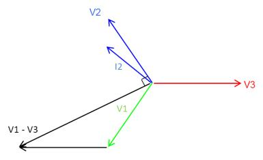
Voltage V3-V1 measurement and measurement of the current on I2
