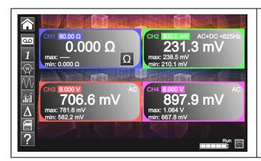
Channel 1 of the *ScopiX* is named CH1. It measures various physical quantities in addition to the signal amplitude measurements, using the appropriate *Probix* accessories. The other channels are voltmeter channels only (or current channels, when used with a *Probix* clamp).
