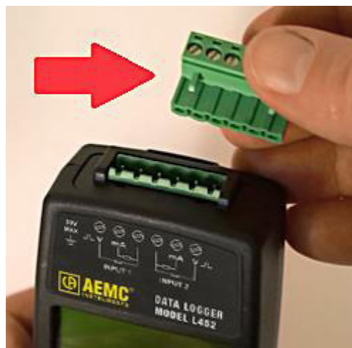
Figure 23. Terminal strip (upper right)
