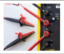
For the probes with Red/Blk and Red/Blk leads and Red DOT located on the probe tip: Connect them as shown here.
