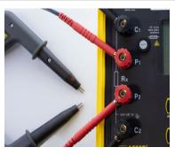
\*For Models 6240 and 6255 instruments with serial numbers lower than 1166339SEDV, terminals C1 and P1 are red, and C2 and P2 are black. In this case, connect probes as shown in the table on the following page.
