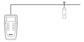
Pressing the TDR / ••••) button will inject a warbling (oscillating) tone into the cable or link under test. When set, the following will be displayed:
