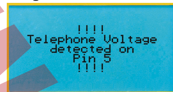
Automatic detection of live telephone voltage.
