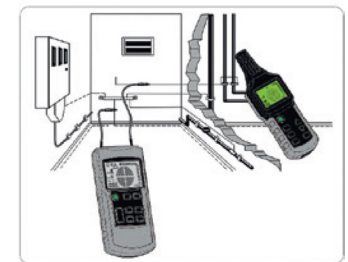
Detection of metal heating ducts and water pipes
