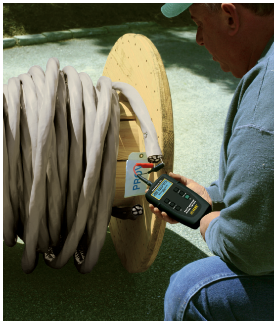
Model CA7024 is used to check length of a power cable on a reel.
