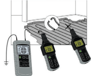
Fault detection in radiant heating systems
