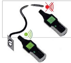
Identification of the network voltage and detection of breaks in the wiring
