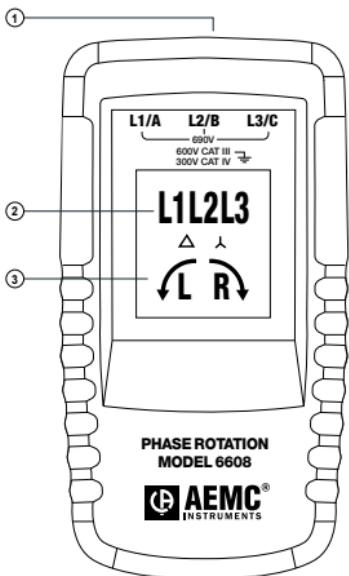
1. Test lead input terminals
