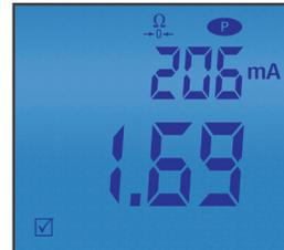
Continuity Measurement and test current Red Backlight and X indicates Alarm (Fail) Condition
