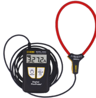
MINIFLEX®: 4000D-14 (14 in probe)
