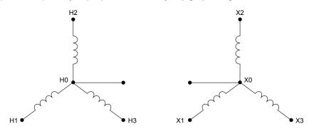
For Y configurations, you must measure from each phase to neutral and from each phase to other phases.
