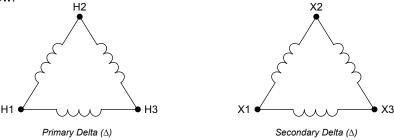
For Delta configurations, you must measure from each phase to other phases. Note that in this configuration, if one coil is open, the Model 8505 can still perform tests because the other two coils may be intact and there is a complete pathway.
