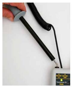
Insert the probe into the terminal labeled SELF TEST (C), and press TEST. The green Capacitor (C) PASS light should blink, and the buzzer should sound.
