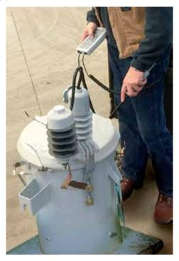
In each test, if the coil is functioning the green Transformer (T) PASS light blinks and the buzzer sounds. (Note that this center tap is sometimes switched in and out.)
