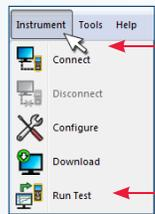
Two easy clicks (Instrument > Run Test) start test and graphs results
