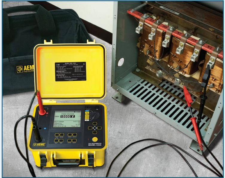
Model 6555 performing an insulation test.
