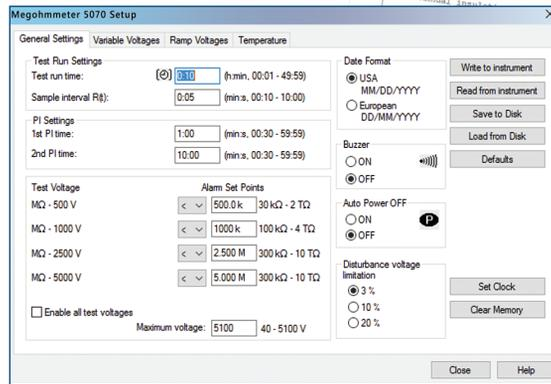
Model 5070 includes Step Function which allows programming of three different test profiles, each containing up to five voltage steps between 40 and 5100V and time per step of up to 10 hours.
