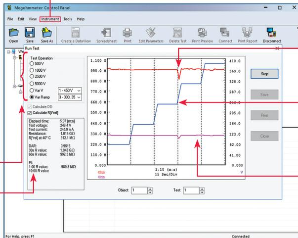
Insulation resistance during the test run
