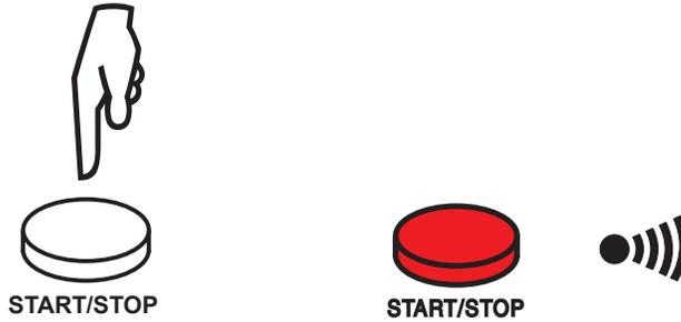
If the test voltage generated is  $>5000V$ , the **START/STOP** button blinks.
