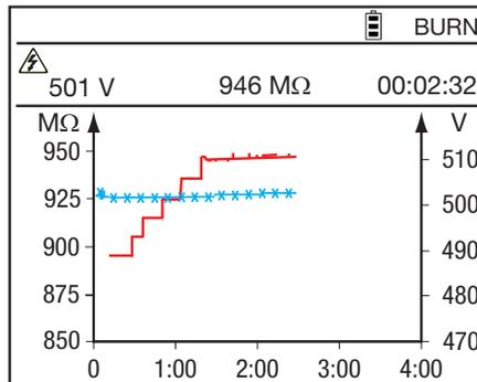
For V-VAR and V-FIXED it is also possible to change measurement parameters during the measurement, by pressing the **CONFIG** button. It is possible to fix the measurement range of the current, to add an analog filter (disturbance level low/high), or to change the test voltage if in the variable test voltage mode (V-VAR). For more details, refer to § 2.4.3.
