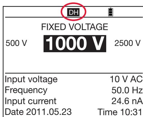
The High setting is recommended when measurements are made in the presence of strong electromagnetic fields at the network frequency (for example near high-voltage lines).
