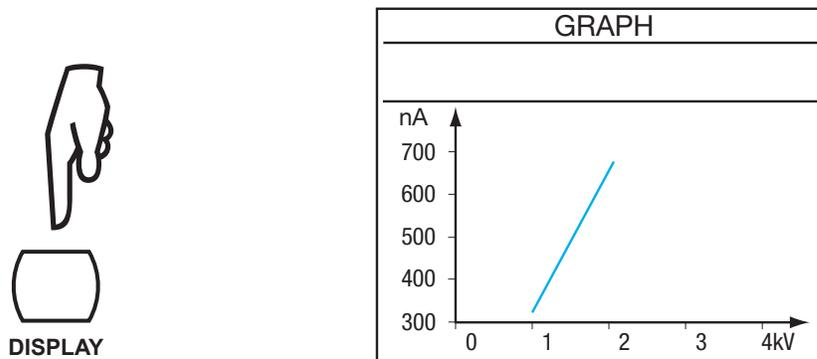
This curve is useful primarily in the case of a measurement in V-RAMP mode.
