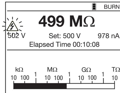
Press the **START/STOP** button again to stop the measurement.
