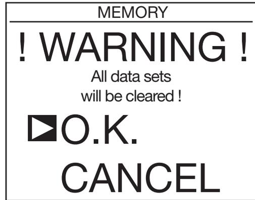
The instrument in this case completely reformats the memory, which takes a few minutes. During this time, it displays “**WAIT**”.
