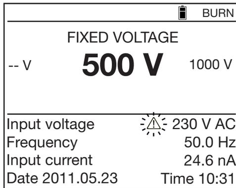
When the external voltage exceeds 25V, the blinking (
