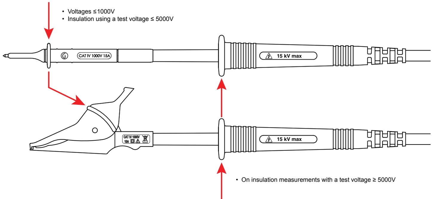
Measurements of voltages  $\geq 1000V$  on supply lines should be made using the test probes only, with the user's hands behind the hand guard on the lead.
