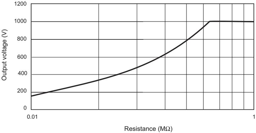
Typical changes in test voltages as a function of the load (cont.):
