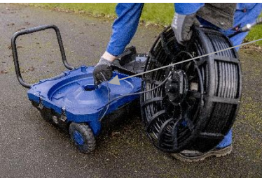
Fig. 98: Pull the connection cable through the opening of the reel holder
