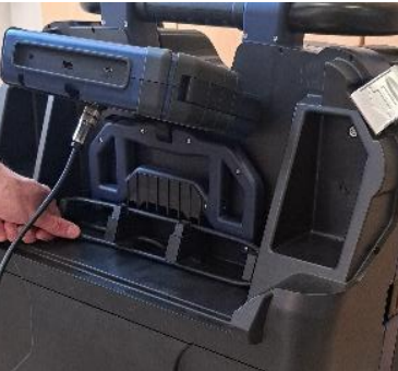
Fig. 103: Wrap the monitor cable around the cable domes
