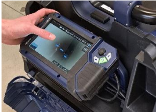
Fig. 74: Set the start and end point of the measuring section.
