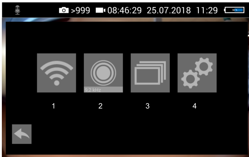
Fig. 54: System menu with the submenus WLAN (1), Locating (2), Picture and video gallery (3) and Settings (4)
