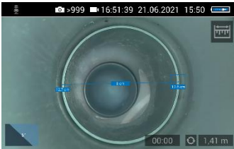
Fig. 67: Display of the distance between two measuring points
