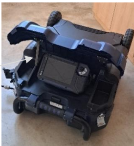
Fig. 35: Wöhler VIS 750 HD inspection camera in horizontal position with glare shield
