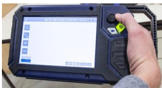
Fig. 33: When the handle is extended, the monitor can be held and operated with one hand.
