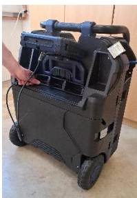
Fig. 32: Roll up the connection cable before pushing the monitor back in.
