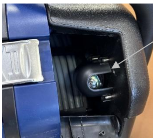
Fig. 22: Transport lock on the camera head
