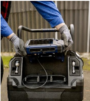
Fig. 89: Pull up the monitor to remove it and the stand from the holder
