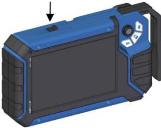
Fig. 34: Push button for pulling out the handle marked with an arrow
