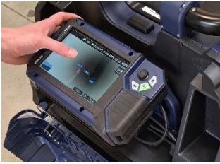
Fig. 69: The measuring points can be moved by dragging
