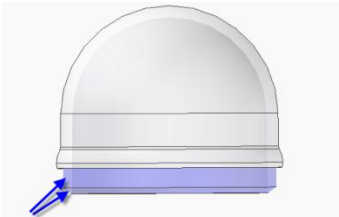
Fig. 87: Installing the camera dome
