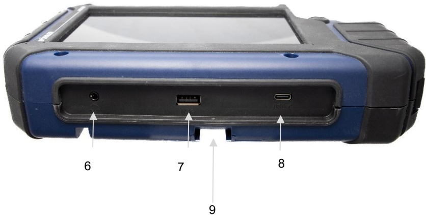
Fig. 9: Monitor underside with connection strip
