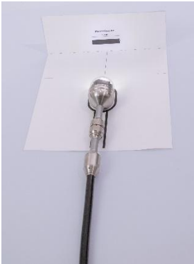
Fig. 71: Calibration with calibration template
