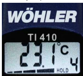
Fig. 5: Bar indication Hold function
