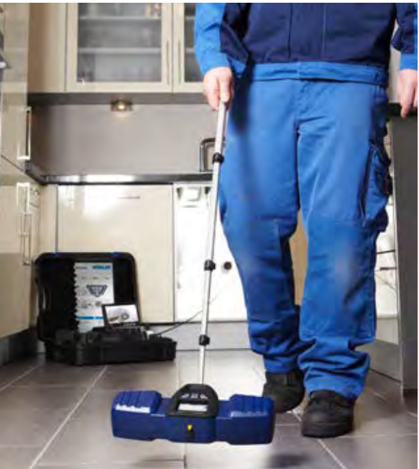
The actual distance count and the position of the head are displayed in the monitor. The Wöhler L 200 Locator makes it possible to locate the camera head.
