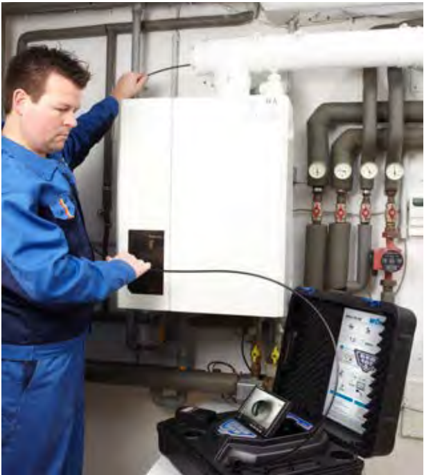
The Wöhler VIS 200 series camera is a valuable tool in a wide range of applications including the analysis of flue gas installations.
