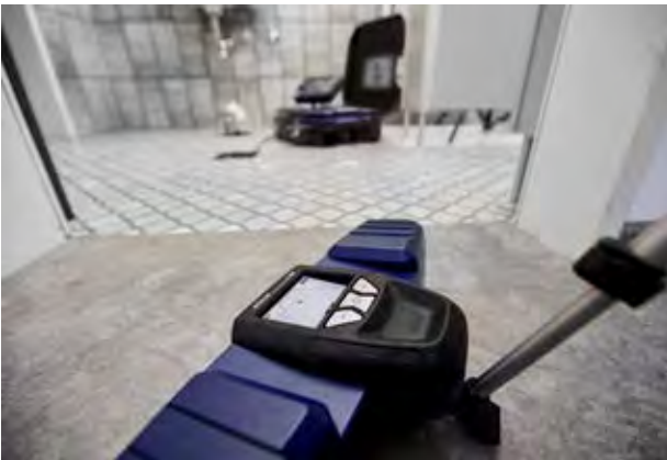
Precise location of the camera head with the Wöhler L 200 Locator.
