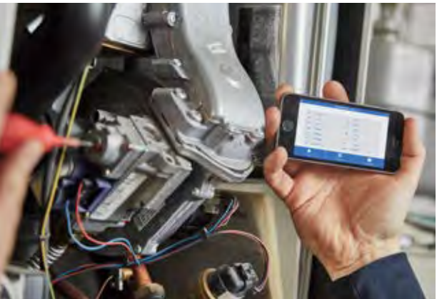
Wöhler Flue Gas Analysis App: Displaying the measured data on a mobile device.
