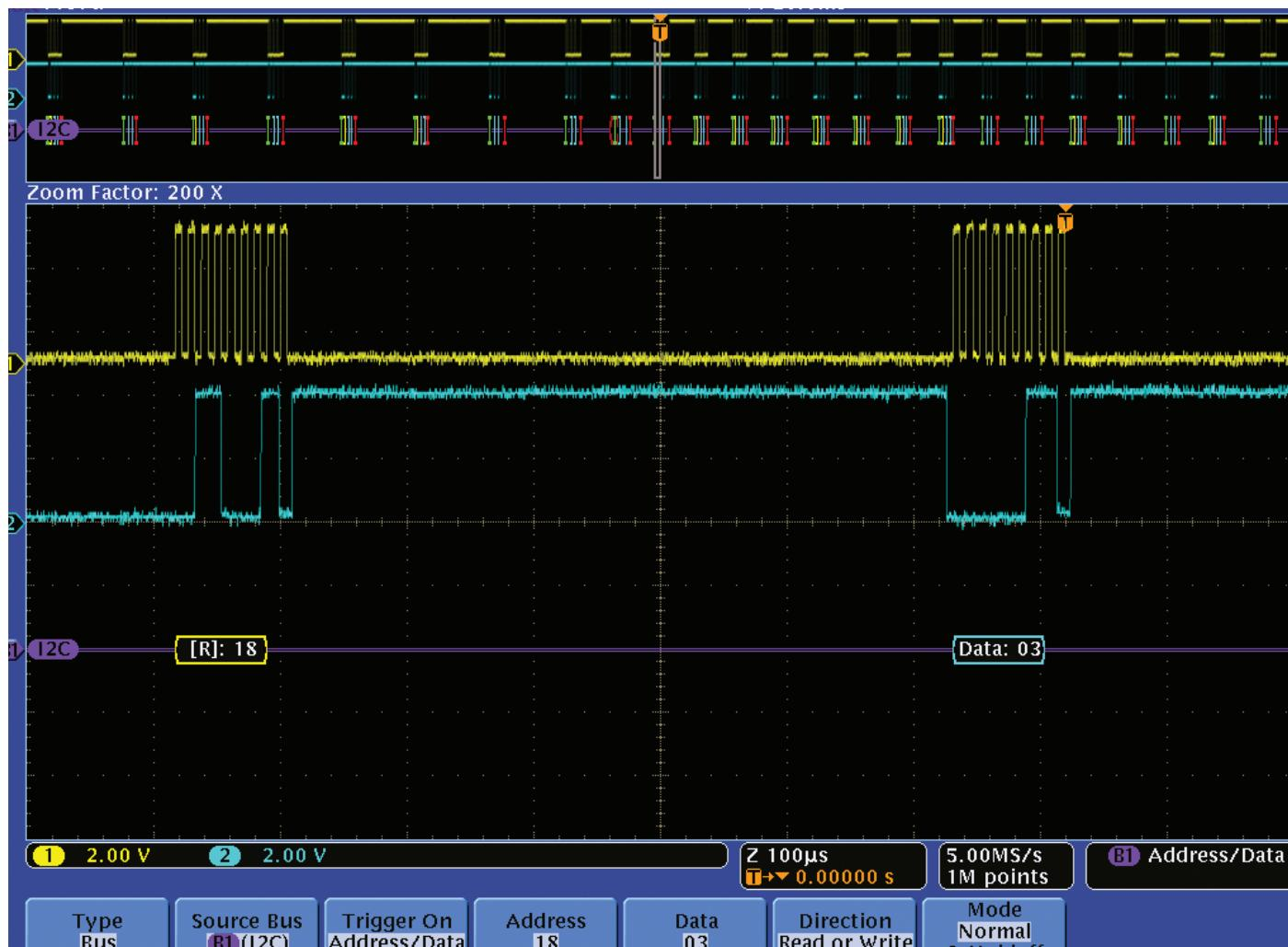
Figure 2. Navigating through a long acquisition of an I<sup>2</sup>C bus.
