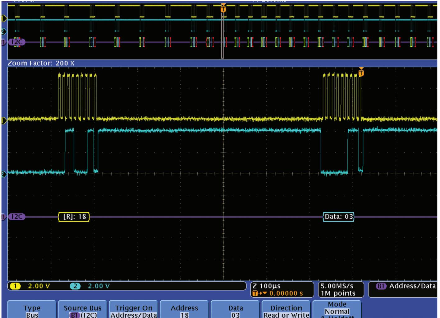
Figure 2. Navigating through a long acquisition of an I2C bus.
