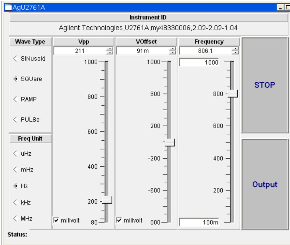
Figure 4.0: Peak to peak voltage and offset voltage in milivolt unit. The range of slider will also change.
