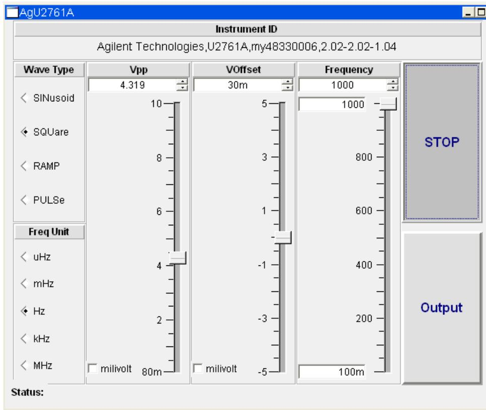
Figure 1.0: A snapshot of the main panel with select Square Waveform signal generation.
