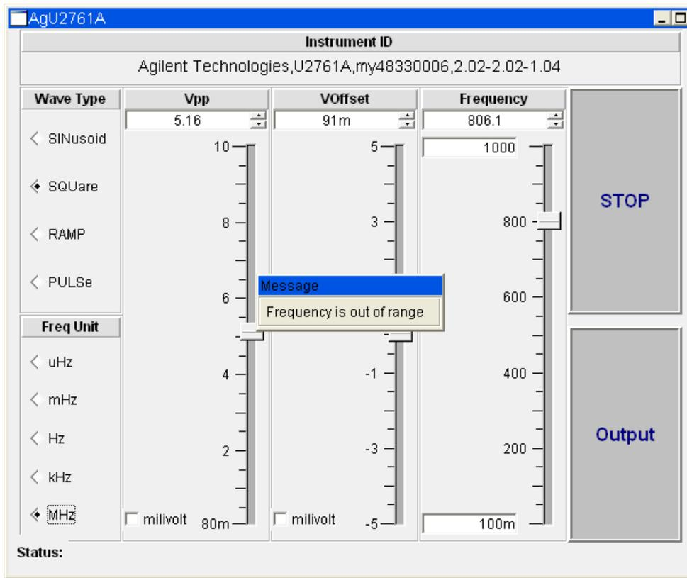
Figure 3.0: In the event of a frequency setting that is out of limits, an error message will appear and the command will not be sent to the instrument.
