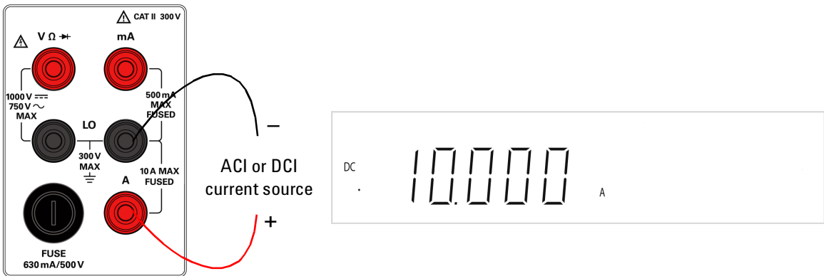
Figure 2-4 ACI RMS or DCI (10A) terminal connection and display
