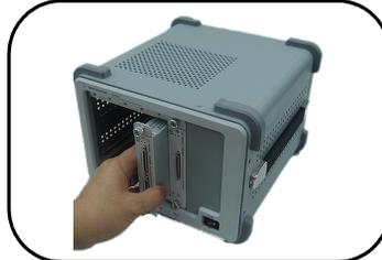
**5** Your USB module is now ready to be plug into an instrument chassis.
