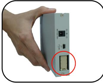
**4** To slot in the USB module to your chassis, turn your USB module perpendicularly and ensure that the 55-pin backplane connector is at the bottom side of the USB module.
