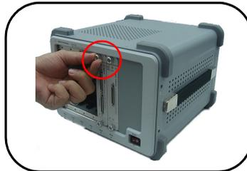
**6** Screw L-Mount Kit to U2781A chassis after USB modular is plugged in.
