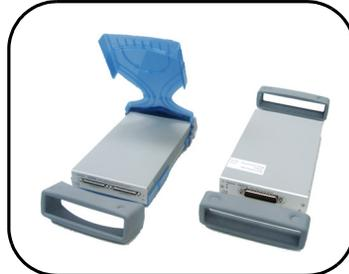
**2** Remove your USB module by pulling the bumper (front end of the casing) in an outward direction. For U2300A, U2500A, and U2600A Series DAQ, lift the plastic body casing and remove it from your USB module.
