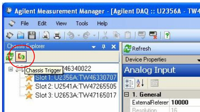
[1] U2781A offers star trigger bus that aims to provide high performance synchronization features that can be configured via Agilent Measurement Manager.
