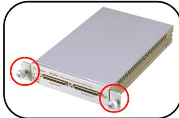
**3** Using the Philip screw driver, screw the L-Mount kit to your USB module.
