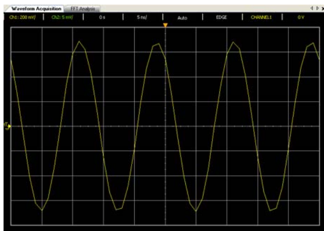
Figure 2-17 The waveform before interpolation
