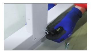
STEP FOUR: Attach lower depth kit rails to legs using M8 hardware. Insert the threaded nut plate into telescoping leg. M8 bolts with washers will hold depth kit rail, leg tube and telescoping leg together.
