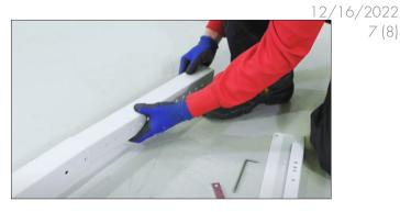
**STEP TWO:** Insert telescoping legs into leg tubes. Align holes with outer side of the leg tubes. Set to desired position/height of the table - remember to include glides and work surface in total height.
