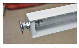
**STEP SEVEN:** Insert glide into bottom of telescoping leg tubes. Attach second nut to glide stem and tighten. (In the above photo, the glide is placed in the shortest position.) If using casters, glide hardware is not needed.
