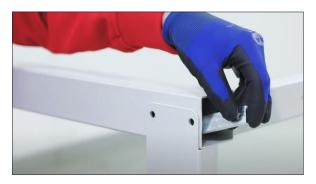
**STEP SIX:** Attach front leg/front rail assembly to the rest of the frame with M8 hardware and nut plates. Insert telescoping legs into leg tubes before attaching lower depth kit rails. (see steps 1-4). Tighten all bolts.
